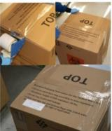
Tape top end-to-end, with reinforcing tape in same manner as bottom. Affix RMW label to top.
